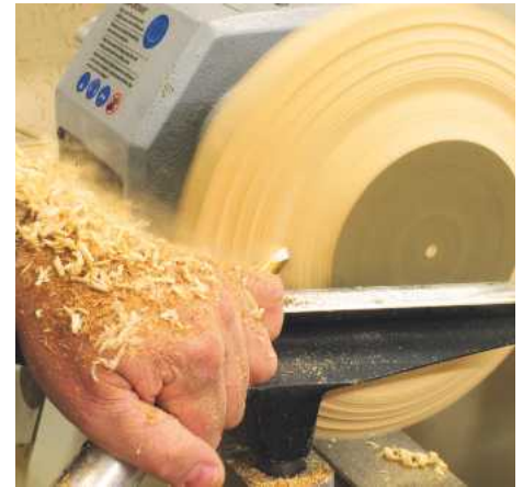
▲ Pic.3 The bigger tool is used for pull cutting and will remove lots of material. To get the best from this tool keep the flute slightly open and the handle down
